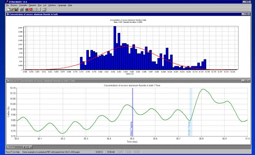
In addition of the irregular  $AlF_3$  addition, the excess  $AlF_3$  concentration variation is influenced by thermal events affecting the  $AlF_3$  evolution like the bath temperature but more importantly by the ledge thickness variation. Figure above shows the daily variation of the concentration of  $AlF_3$  in the bath in absence of control and any  $AlF_3$  mass imbalance. The standard deviation on the average value is about 0.1%.
