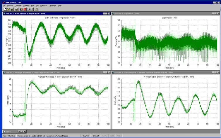
Figure above presents the results obtained using the standard control described above. After the change of superheat, the 970 °C temperature target is no longer compatible with the 10% excess  $AlF_3$  target, this combined with the 1 day offset between the  $AlF_3$  feedback and the temperature feedback generates a cyclic response characteristic of somewhat unstable feedback control.
