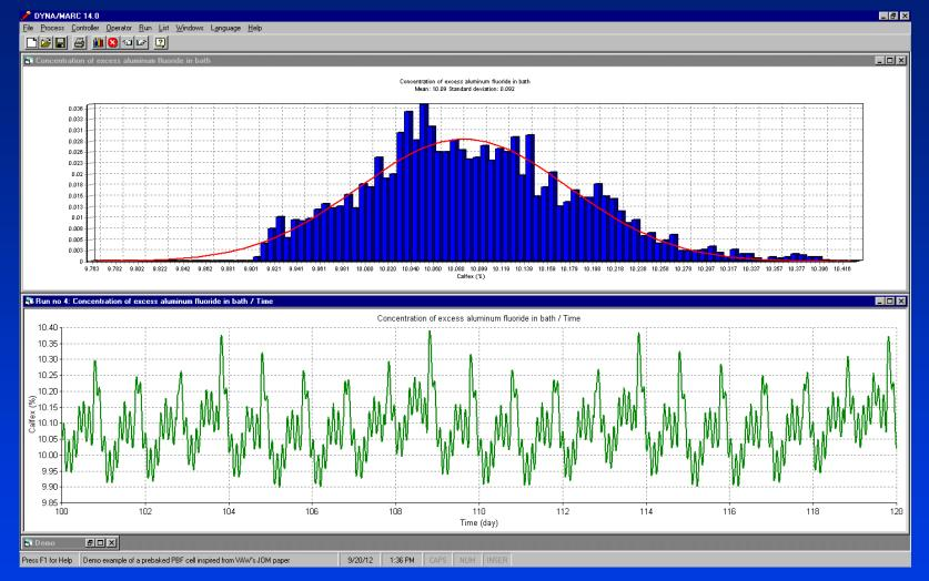
Figure above shows the variation of the  $AIF_3$  for a period of 20 days again without control and any mass imbalance.
