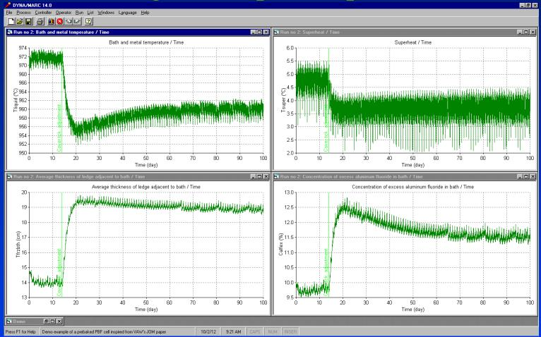
As we can see in figure above, as a natural response, the cell must reduce its cathode heat loss of the same amount by reducing its superheat by about 1 °C and increasing its ledge thickness by about 5 cm. As a result, of this extra ledge formation, the excess  $AIF_3$  increase by about 2% and remains close to 12% if the direct  $AIF_3$  additions remain unchanged.
