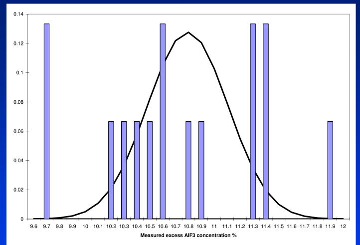
Figure above highlights the relative variability or lack of strict repetitivity of the measurements which in turn highlight the lack of homogeneity of the bath. The standard deviation of that bath sampling noise has been evaluated to be around 0.5 % which is 5 times greater than the process noise generated by daily events (ref: ICSOBA 2012).
