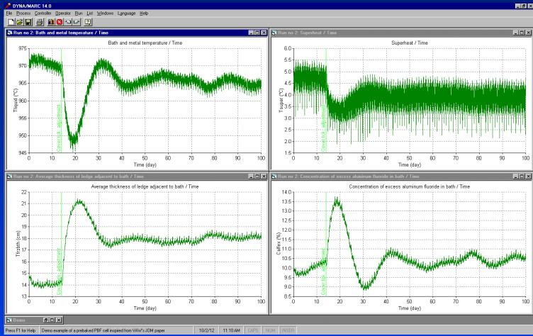
Simulation of the process with a significant perturbation; feedback control, 10% target concentration: STARprobe<sup>TM</sup> measurements once per day, 0.5 kg/hr% proportional band and daily 0.1 micro-ohm target resistance correction due to superheat offset from target.
